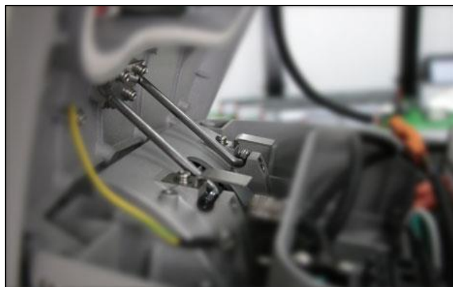
Maintaining the opening of the cover is ensured and secured by a self-locking rod
